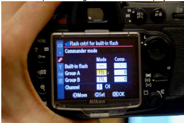
5. Make sure that you have selected “Channel 3” and that group A is set to TTL (Through-The-Lens) Metering.
