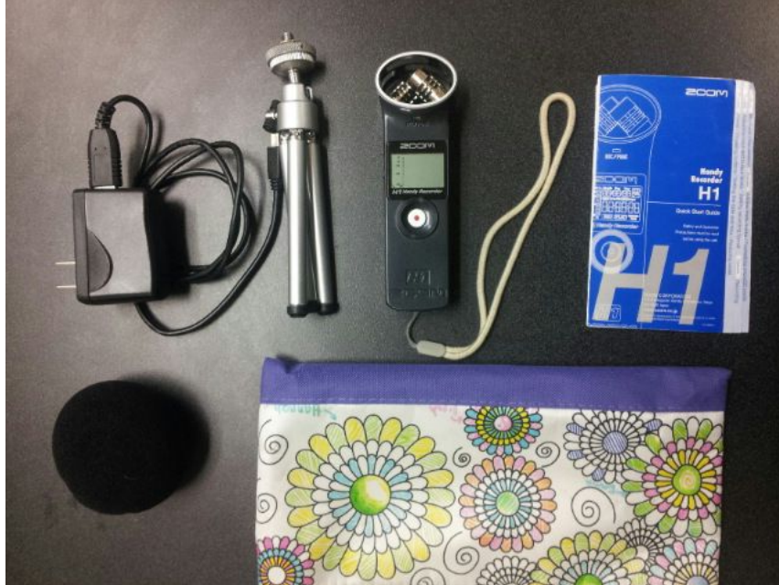
This is a ZOOM H1 recorder kit. It accepts \frac{1}{8} " inputs, or can be used as a stand alone stereo recorder. In the bottom left of the picture is a windshield that fits over the built in mics. In the top left corner is an A/C wall charger that allows the unit to run off 110V. To the right of the charger is a tripod to mount the ZOOM on.
