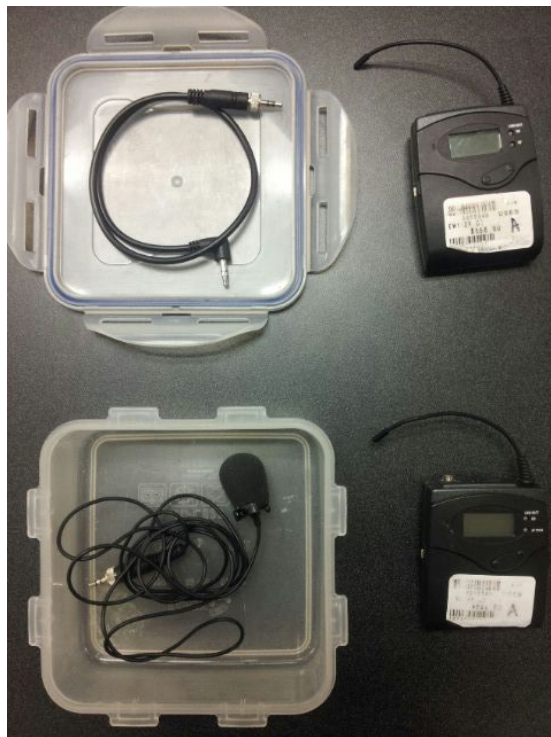
This picture shows a Lavallier microphone in the bottom left. It gets clipped onto a lapel and runs to the wireless transmitter to the right of it. The mic and receiver is attached to the actor. It sends a signal to the receiver that is pictured in the top right corner.
